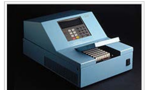
"Baby Blue", a 1986 prototype machine for doing PCR
