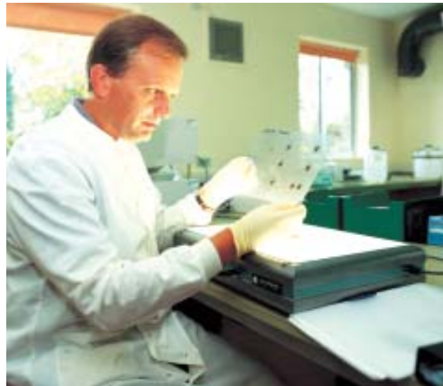
Scrapie testing using the Prionics-check technique (a western immunoblotting system)
