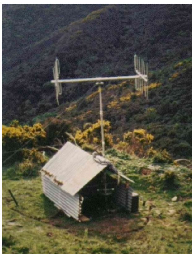
Figure 2.3 Radio triangulation site
